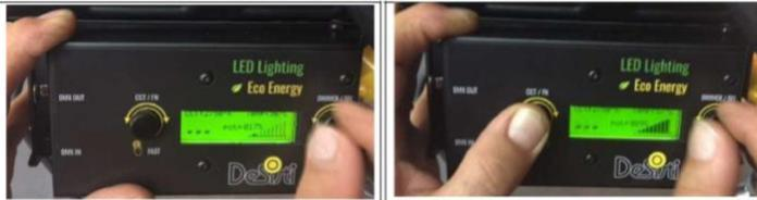
When the DISPLAY is in STAND BY Mode, please rotate KNOB 2 to act on the LIGHT INTENSITY Dimming...Clock Wise to increase the level and Counter Clock Wise to decrease it. Fine control: 1 full TURN of the KNOB 2 = 5% Dimming Variation
