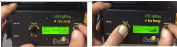
When the DISPLAY is in STAND BY Mode, please rotate KNOB 2 to act on the LIGHT INTENSITY Dimming...Clock Wise to increase the level and Counter Clock Wise to decrease it. Fine control.
