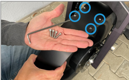
The fender for the front is mounted with 4 screws.
