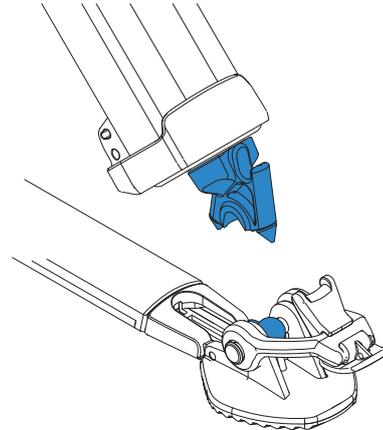
3. Bend the rubber strap **1** and engage the bottom edge of the lever in the tripod recess.
