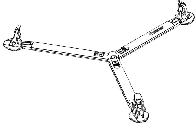
2. Place the tripod foot on the ball of the spreader foot.
