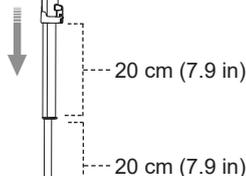
3. With an average downward force of 20 - 30 kg (44 - 66 lb) **flowtech 75** or 30 - 40 kg (66 - 88 lb) **flowtech 100** applied, the leg should remain extended.
