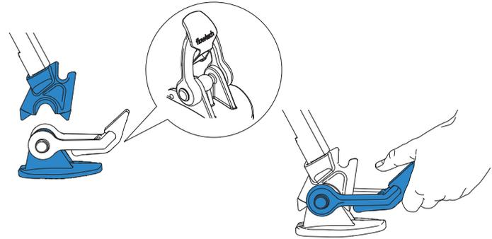
2. Bend the rubber strap **1** and engage the bottom edge of the lever in the tripod recess.
