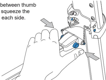
2. Align the latching pins with the locating holes on the tripod leg.
