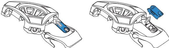
4. Lift out the hinge lock button.
