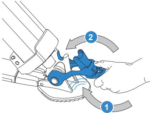
5. Tripod spiked foot secured in the Ground Spreader Foot.
