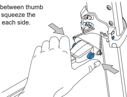
2. Align the latching pins with the locating holes on the tripod leg.
