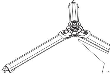
3. Use a torque screwdriver to adjust the M5 screws to the correct torque. (2.5Nm to 3.5Nm Max)
